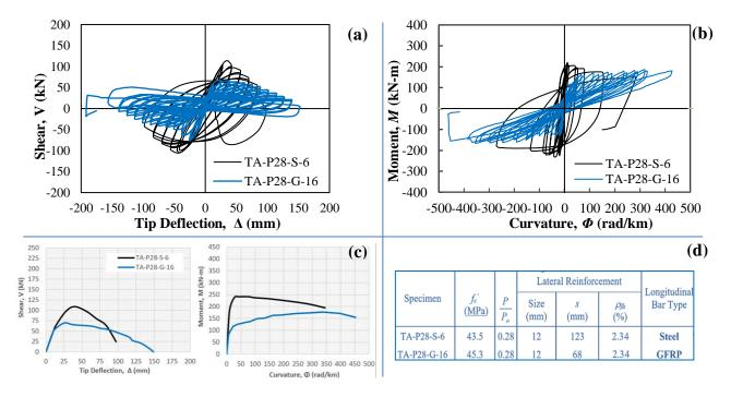
Figure 7. Effect of Longitudinal Bar Type: (a)  $V-\delta$  hysteresis response, (b)  $M-\phi$  hysteresis response, (c) envelope curves, and (d) specimen details
