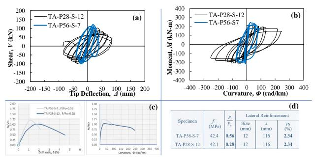
Figure 4. Effect of Axial Load Level: (a) V– $\delta$  hysteresis response, (b) M– $\phi$  hysteresis response, (c) envelope curves, and (d) specimen details
