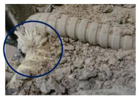
Figure 6. Crushing of GFRP longitudinal bar in Specimen 16
