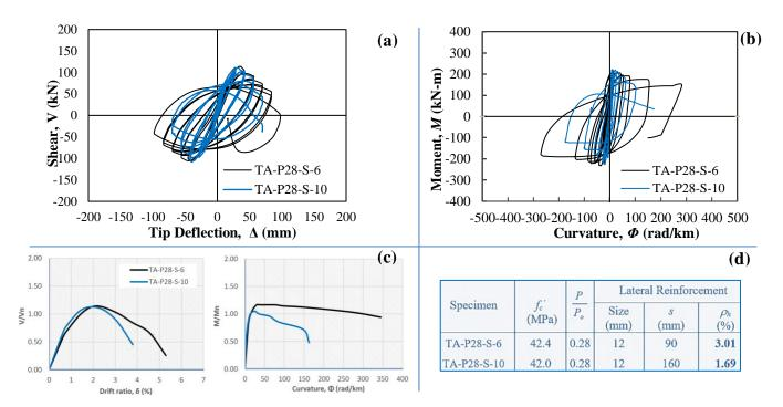
Figure 5. Effect of amount of lateral reinforcement: (a) V– $\delta$  hysteresis response, (b) M– $\phi$  hysteresis response, (c) envelope curves, and (d) specimen details
