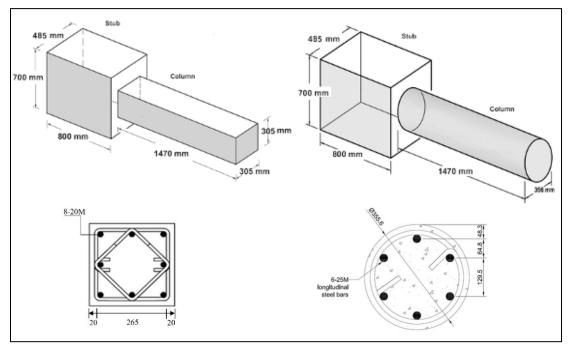
Figure 1: Geometry of specimens: (a) circular, and (b) square
