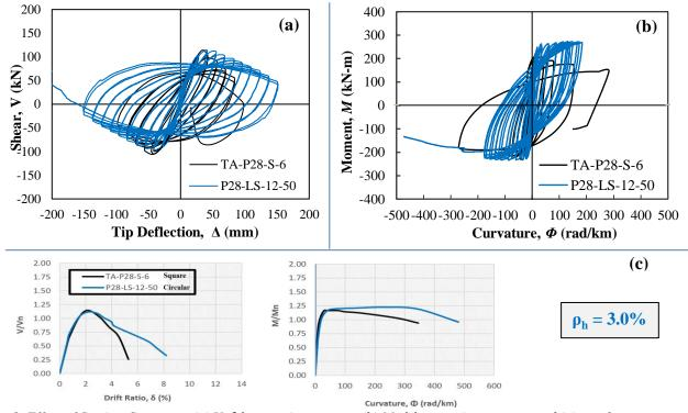
Figure 9. Effect of Section Geometry: (a) V-δ hysteresis response, (b) M-φ hysteresis response, and (c) envelope curves
