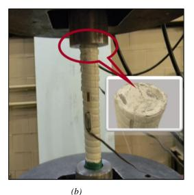
Figure 3. Failure Modes of the GFRP Coupons in: (a) tension, and (b) compression.
